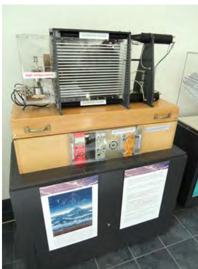
Figure 19.6 A spark chamber is used to trace the paths of high-energy particles. Ionization created by the particles as they pass through the gas between the plates allows a spark to jump. The sparks are perpendicular to the plates, following electric field lines between them. The potential difference between adjacent plates is not high enough to cause sparks without the ionization produced by particles from accelerator experiments (or cosmic rays). (credit: Daderot, Wikimedia Commons)
