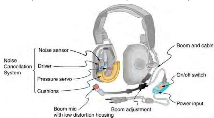
Figure 17.22 Headphones designed to cancel noise with destructive interference create a sound wave exactly opposite to the incoming sound. These headphones can be more effective than the simple passive attenuation used in most ear protection. Such headphones were used on the record-setting, around the world nonstop flight of the Voyager aircraft to protect the pilots’ hearing from engine noise.
