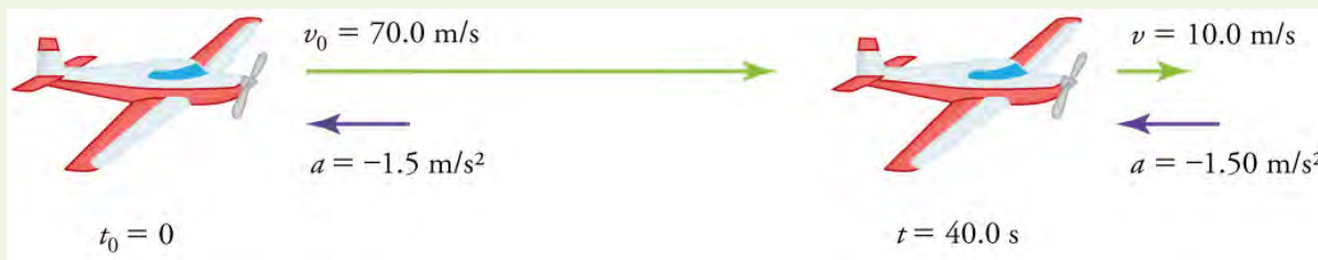
Figure 2.29 The airplane lands with an initial velocity of 70.0 m/s and slows to a final velocity of 10.0 m/s before heading for the terminal. Note that the acceleration is negative because its direction is opposite to its velocity, which is positive.
