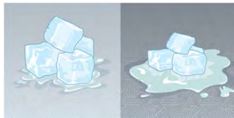
Figure 14.25 This illustration shows that the darker pavement is hotter than the lighter pavement (much more of the ice on the right has melted), although both have been in the sunlight for the same time. The thermal conductivities of the pavements are the same.
