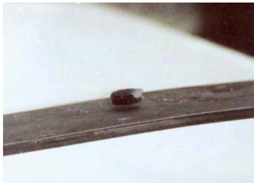
Figure 34.24 One characteristic of a superconductor is that it excludes magnetic flux and, thus, repels other magnets. The small magnet levitated above a high-temperature superconductor, which is cooled by liquid nitrogen, gives evidence that the material is superconducting. When the material warms and becomes conducting, magnetic flux can penetrate it, and the magnet will rest upon it. (credit: Saperaud)
