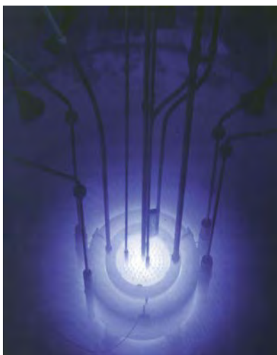
Figure 17.20 The blue glow in this research reactor pool is Cerenkov radiation caused by subatomic particles traveling faster than the speed of light in water. (credit: U.S. Nuclear Regulatory Commission)
