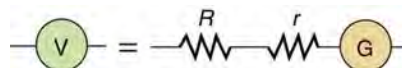
Figure 21.29 A large resistance R placed in series with a galvanometer G produces a voltmeter, the full-scale deflection of which depends on the choice of R . The larger the voltage to be measured, the larger R must be. (Note that r represents the internal resistance of the galvanometer.)
