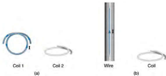
Figure 23.56 (a) The planes of the two coils are perpendicular. (b) The wire is perpendicular to the plane of the coil.
