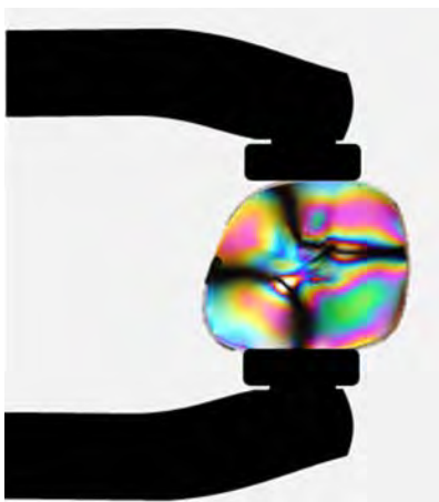
Figure 27.49 Optical stress analysis of a plastic lens placed between crossed polarizers. (credit: Infopro, Wikimedia Commons)
